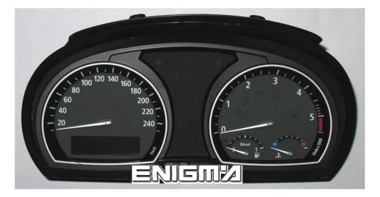
Use cable C4, open all dash, please make it carefully, then locate eprom memory M35080, we don't need to desolder it, and clip it checking pin 1 as shown of photo below:
