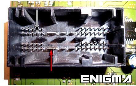
AND THEN CONNECT OR SOLDER CABLE LEADS ACCORDING TO POITNS SHOWN INTO PHOTO:
