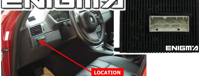
USE CABLE C12, REMOVE MODULE FROM CAR, OPEN COMPLETELY IT, WHEN WE HAVE BOARD ON OUR HANDS, FIRST CONNECT POWER LEADS:
