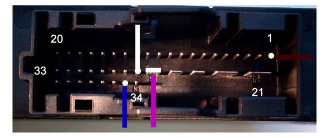
CAS PIN 25 - ENIGMA DB25 PIN 03 GND CAS PIN 35 - ENIGMA DB25 PIN 08 CAN CAS PIN 26 - ENIGMA DB25 PIN 21 CAN CAS PIN 01 - ENIGMA DB25 PIN 25 +12V 2. USE CABLE C45 + A6 ADAPTER. REMOVE MODULE FROM CAR CAREFULLY, OPEN IT, LOCATE POINTS ON BOTH SIDES FROM BOARD AND SOLDER CABLE LEADS:
