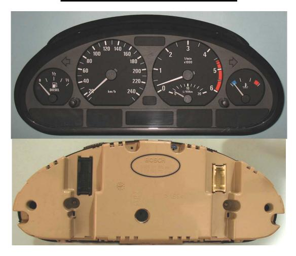
USE CABLE C4, OPEN ALL DASH, PLEASE MAKE IT CAREFULLY, THEN LOCATE EPROM MEMORY, AND CLIP IT CHECKING PIN 1 AS SHOWN OF PHOTO BELOW:
