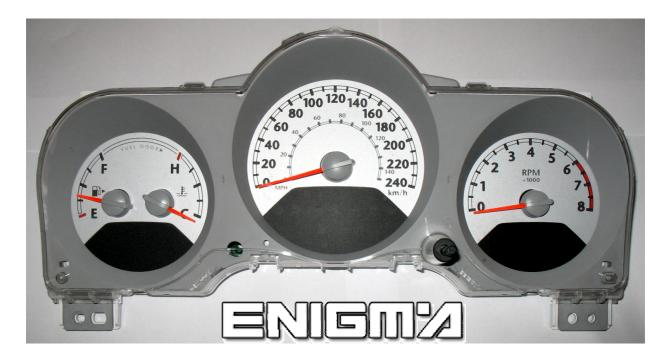
USE CABLE C4, OPEN BACK PART OF DASH, CAREFULLY, THEN LOCATE MEMORY, A RL76 EPROM, AND CLIP IT CHECKING PIN 1 AS SHOWN OF PHOTO BELOW:
