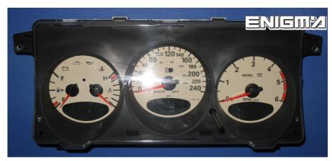
USE CABLE C12 O HCS12, REMOVE BACK COVER FROM DASH, THEN CONNECT POWER LEADS LIKE WE CAN SEE ON THIS PHOTO:
