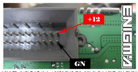
CONNECT OR SOLDER CABLE LEADS ACORDING TO COLOURS LIKE ON THIS PHOTO:
