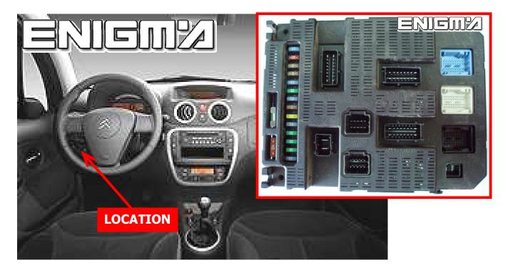
USE CABLE C7, REMOVE BACK PLASTIC COVER FROM BSI, THEN CONNECT OR SOLDER CABLE LEADS ACCORDING TO PIN AS SHOWN OF BELOW PHOTO:
