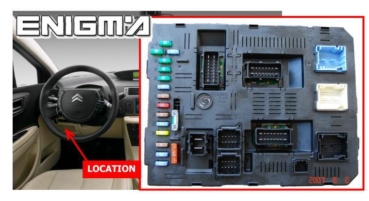
USE CABLE C4, REMOVE BACK PLASTIC COVER FROM BSI, THEN LOCATE EEPROM MEMORY AND CLIP IT CHECKING PIN 1 AS SHOWN OF PHOTO BELOW:
