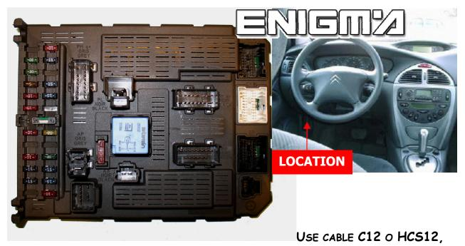
REMOVE BACK PLASTIC COVER FROM **BSI**, THEN CONNECT OR SOLDER CABLE LEADS ACCORDING TO COLOURS AS SHOWN OF BELOW PHOTO:
