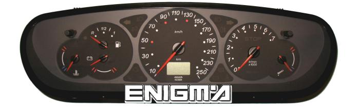
Use cable C12, remove back cover from dash, then connect or solder cable leads according to colours as shown of below photo during 30 seconds:
