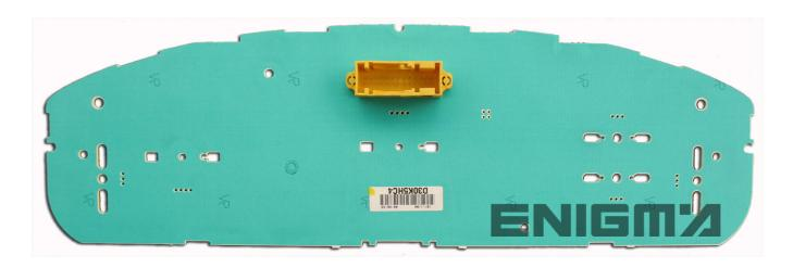
USE CABLE C12, TAKE OFF CAREFULLY NAILS (TO CONNECT MAKE IT WITH POWER), AND ALL PLASTICS TILL WE HAVE CLEAN THE BOARD, NOW SOLDER CABLE LEADS ACCORDING TO COLOURS AS SHOWN OF BELOW PHOTO:
