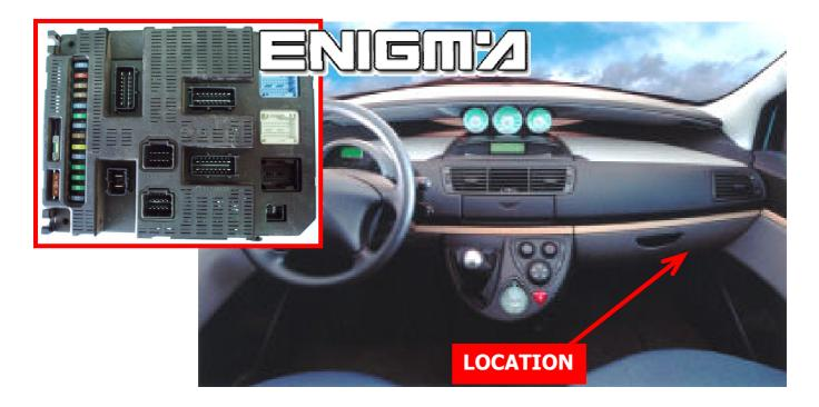
USE CABLE C7, REMOVE BACK PLASTIC COVER FROM BSI, THEN CONNECT OR SOLDER CABLE LEADS ACCORDING TO PIN AS SHOWN OF BELOW PHOTO:
