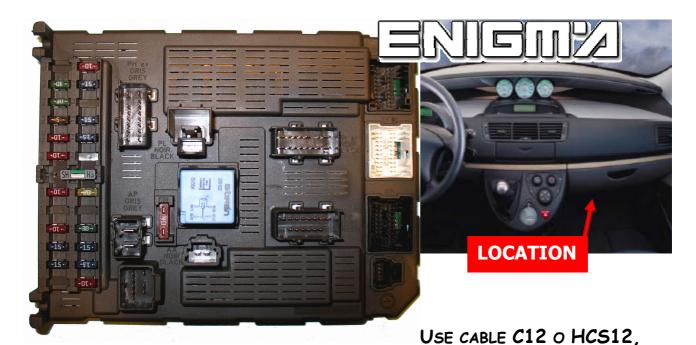
REMOVE BACK PLASTIC COVER FROM **BSI**, THEN CONNECT OR SOLDER CABLE LEADS ACCORDING TO COLOURS AS SHOWN OF BELOW PHOTO:
