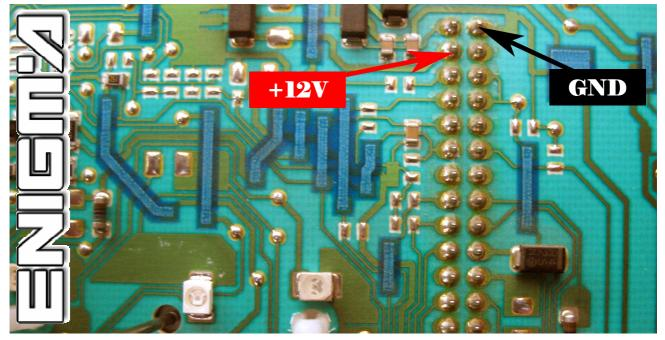
CONNECT OR SOLDER CABLE LEADS ACORDING TO COLOURS AS SHOWN OF BELOW PHOTO, DON'T FORGET TO REALIZE A BRIDGE BETWEEN POINTS:
