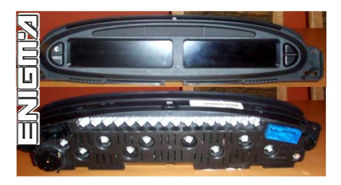
USE CABLE C4, OPEN BACK PART OF DASH, CAREFULLY, DON'T TOUSH SCREENS AT ANY TIME, THEN LOCATE EPROM 93C66 MEMORY, AND CLIP IT CHECKING PIN 1 AS SHOWN OF BELOW PHOTO:
