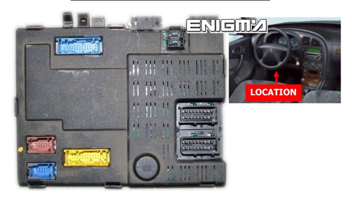
USE CABLE C4, OPEN BACK COVER FROM BSI, CAREFULLY, THEN LOCATE EPROM MEMORY 95040, AND CLIP IT CHECKING PIN 1 AS SHOWN OF PHOTO BELOW:
