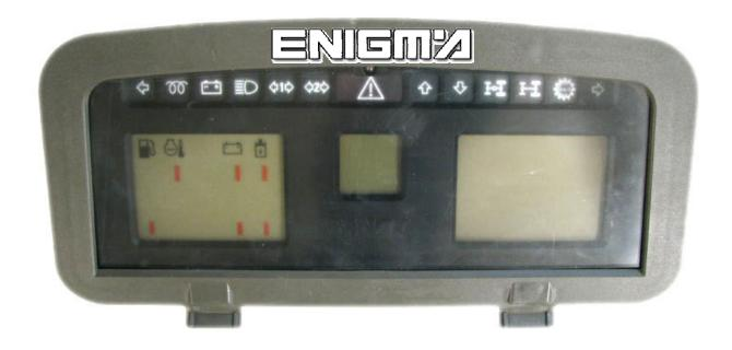
USE CABLE C4, REMOVE BACK PLASTIC COVER FROM DASH, THEN CAREFULLY TURN OUT MAIN BOARD, NOW WE CAN LOCATE EEPROM 93C56 MEMORY AND CLIP IT CHECKING PIN 1 AS SHOWN OF PHOTO BELOW:
