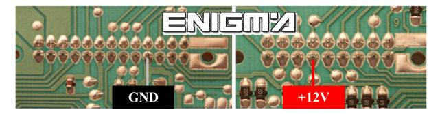
CONNECT OR SOLDER CABLE LEADS ACORDING TO COLOURS AS SHOWN OF PHOTO BELOW, DON'T FORGET TO REALIZE A BRIDGE BETWEEN 2 POINTS:
