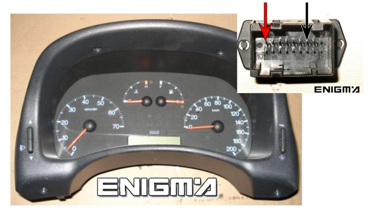
USE CABLE C4, TAKE OFF DASH FROM CAR DASH, OPEN ALL DASH, PLEASE MAKE IT CAREFULLY. WHEN WE HAVE MAIN BOARD ON OUR HANDS LOCATE EPROM MEMORY, AND CLIP IT CHECKING PIN 1 AS SHOWN OF PHOTO BELOW:
