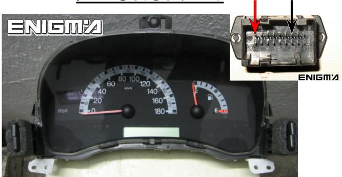
USE SPECIFIC CABLE C39, TAKE OFF DASH FROM CAR, OPEN ALL DASH, PLEASE MAKE IT CAREFULLY, SPECIALLY WITH NAILS. WHEN WE HAVE MAIN BOARD ON OUR HANDS, CONNECT POWER PLUG TO DASH LIKE WE CAN SEE ON PHOTO:
