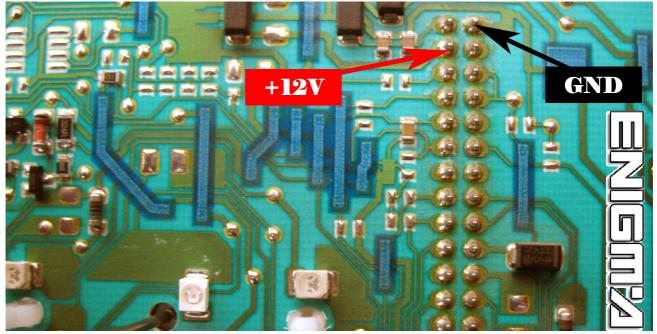
CONNECT OR SOLDER CABLE LEADS ACORDING TO COLOURS AS SHOWN OF BELOW PHOTO, DON'T FORGET TO REALIZE A BRIDGE BETWEEN POINTS:
