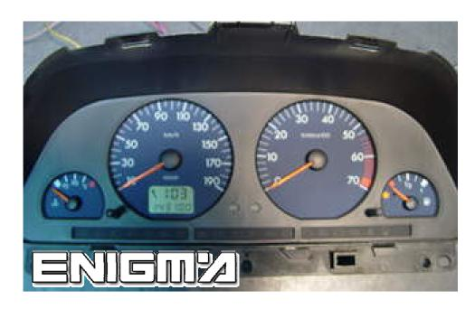
USE SPECIFIC CABLE C20, REMOVE DASH FROM CAR, AND CONNECT PLUG TO DASH LIKE WE CAN SEE ON NEXT PHOTO AND RUN PROGRAM:
