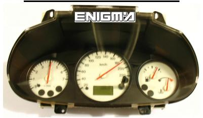
Use specific cable C37, take off from car dash, open back of dash, with 5 torx screws. When back side of board is in front, connect plug to dash like we can see on next photo:
