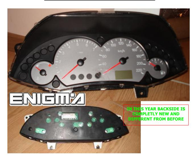
USE CABLE C4, OPEN ALL DASH, PLEASE MAKE IT CAREFULLY, THEN LOCATE EPROM MEMORY, AND CLIP IT CHECKING PIN 1 AS SHOWN OF PHOTO BELOW:
