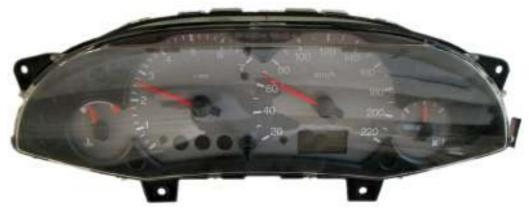
Use specific cable C36, remove dash from car, connect plug into white dash plug, and grey cable to the point show on photo:
