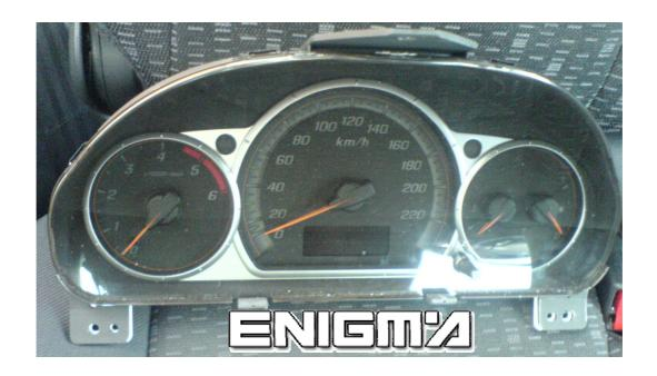
USE CABLE C4, OPEN BACK SIDE OF DASH, CAREFULLY, THEN LOCATE EPROM 93C66 MEMORY, AND CLIP IT CHECKING PIN 1 AS SHOWN OF BELOW PHOTO:
