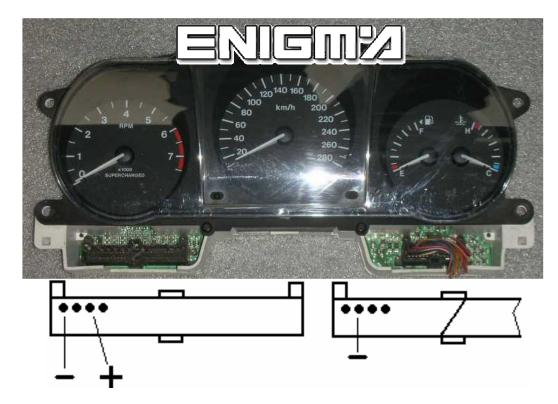
USE CABLE C11, REMOVE BACK COVER FROM DASH, THEN CONNECT OR SOLDER CABLE LEADS ACCORDING TO COLOURS AS SHOWN ON PHOTO, REMEMBER TO LIF UP ONE PIN FROM MICRO:
