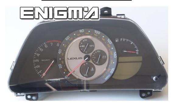
USE C4 CABLE, OPEN REAR PART OF DASH, THEN SOME SCREWS WILL BE APPEARS, NAILS AND YOU WILL HAVE FREE THE MAIN BOARD, THEN LOCATE EPROM MEMORY 93C46, AND CLIP IT CHECKING PIN 1 AS SHOWN OF BELOW PHOTO:
