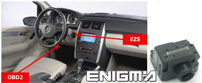
Now remove back plastic cover from EZS, and locate points on the board checking photos belows and solder cable leads as it shows to us: Version 1:
