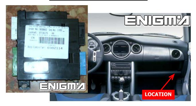
Use cable C4, open back side from BCU, locate eeprom 93C76 memory and clip it checking Pin 1 as shown of photo below:
