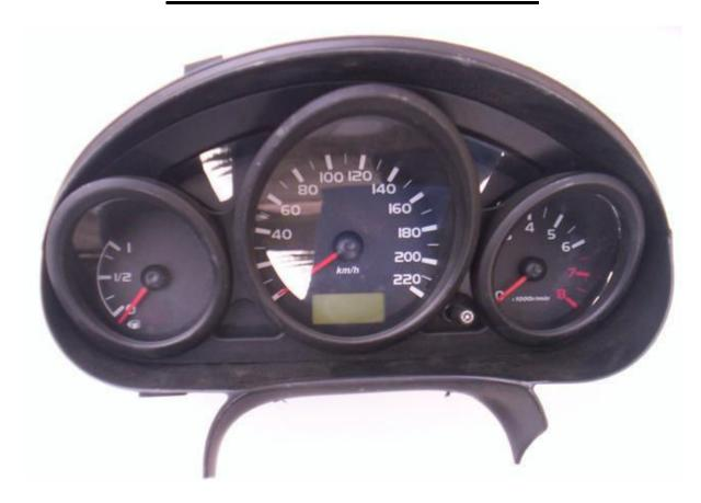
USE C7 CABLE, WE ONLY NEED TO REMOVEFF BACK PLASTIC COVER FROM DASH, LOCATE POINTS IN THE MAIN BOARD LIKE IN PHOTO BELOW AND SOLDER CABLE LEADS AS IT SHOWS TO US. NEVER TOUCH NAILS, IT IS VERY DANGEROUS. MEMORY INSIDE THOSE KIND OF CARS ARE A 93C56 OR LS56.
