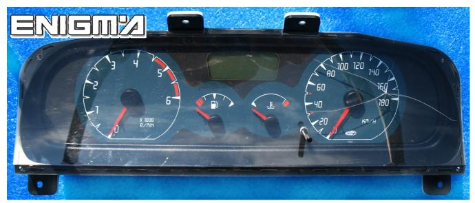
USE CABLE C12, REMOVE DASH FROM CAR, OPEN BACK COVER OF DASH, JUST PULL IT OUT. SOLDER POWER LEADS AND COLOUR LEADS LIKE WE CAN SEE ON NEXT PHOTOS ACCORDING TO COLOURS:
