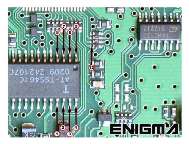
WE MUST DESOLDER RESISTOR FROM LEAD 9 AND UP PIN 10:
