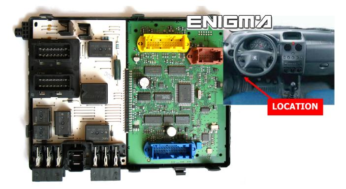
USE CABLE C13 ALWAYS CONNECTED TO A1 ADAPTER. REMOVE BOTH SIDES FROM BSI, THEN CONNECT OR SOLDER CABLE LEADS ACCORDING TO NUMBER AS SHOWN IN NEXT PHOTOS:
