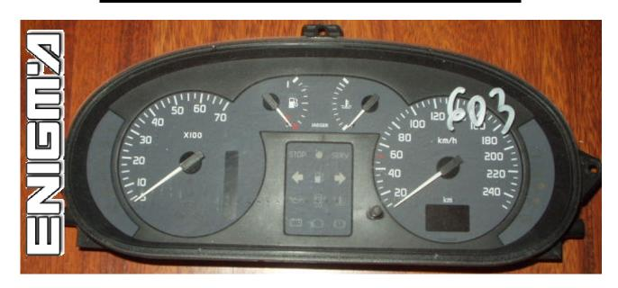
USE CABLE C13 ALWAYS CONNECTED TO A1 ADAPTER. OPEN COMPLETELY DASH, WE MUST REMOVE NAILS, THEY HAVE NO COMPLICATION, THEN CONNECT OR SOLDER CABLE LEADS ACCORDING TO NUMBER AS SHOWN IN NEXT PHOTO:
