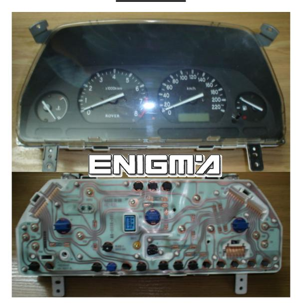
Use cable C4, remove front plastic cover, take off speedometer, only fixing with 4 screws. Then locate eprom memory 93C46, clip it checking pin 1 as shown of photo below:
