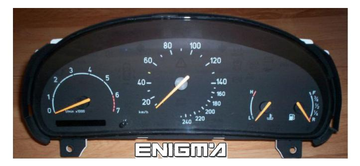
Use cable C4, remove rear plastic cover. Then locate eprom memory 93C46 or S130, sometimes this must be desolder to show new value on display, clip it checking pin 1 as shown of photo below:
