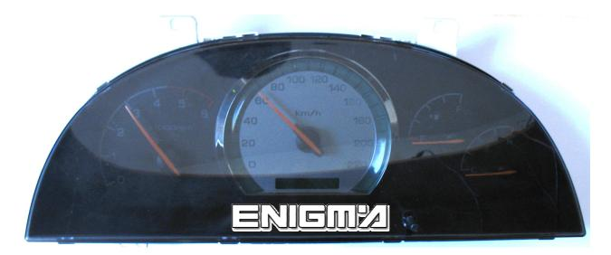
Use cable C4, open back part of dash, carefully, then locate eprom 93C46 memory, and clip it checking pin 1 as shown of below photo:
