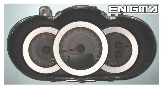
USE **C7** CABLE, REMOVE BACK SIDE OF DASH, PUSH OUT SPEEDOMETER, THEN LOCATE POINTS ON THE MAIN BOARD LIKE IN PHOTO BELOW AND SOLDER CABLE LEADS AS IT SHOWS TO US:
