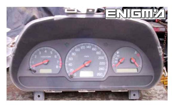
USE C7 CABLE, REMOVE DASH FROM CAR, WE MUST REMOVE OUT PLASTIC COVERS, THEN WE WILL HAVE BOARD WITH NAILS AND ENGINE, USUALLY WE MUST DESOLDER SCREEN, BUT WITH OUR METHOD THIS IS NOT NECESSARY. LOCATE POINTS ON THE BACK SIDE FROM MAIN BOARD LIKE IN PHOTO BELOW AND SOLDER CABLE LEADS AS IT SHOWS TO US:
