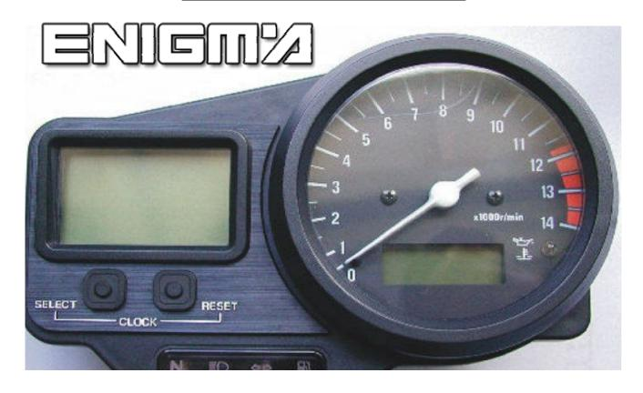
USE CABLE C7, OPEN BACK PART OF DASH, THEN LOCATE POINTS SHOWN OF BELOW PHOTO, AND THEN SOLDER CABLE LEADS CONCORDANCE WITH ITS NUMBER:
