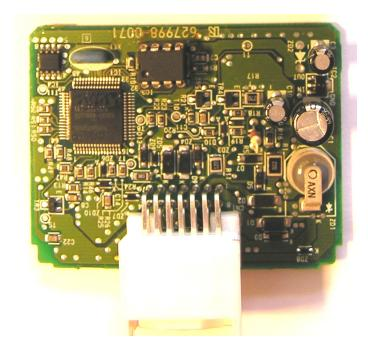
Remove immobiliser ECU from the car and open it. Find 93C66 EEPROM in DIP package. Use **A5** or **A4** adapter and follow CarProg instruction to program transponder key. Short quartz resonator for in-circuit EEPROM programming or remove 93C66 from immobiliser board.
