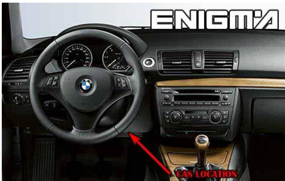
PHOTO 1: Locate the CAS2 module in the car.
