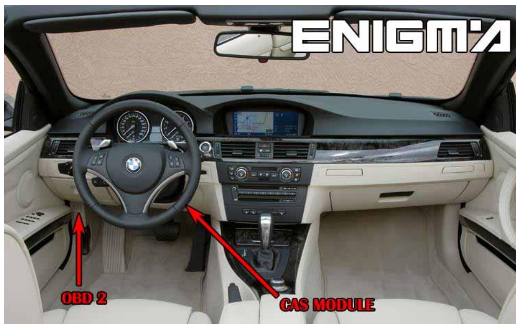
PHOTO 1: Locate the CAS3 module in the car.
