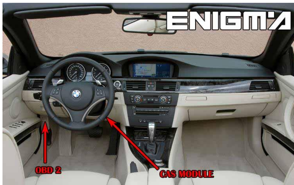
PHOTO 1: Locate the CAS2 module in the car.
