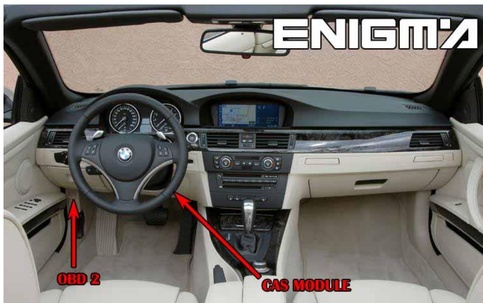
PHOTO 1: Locate the CAS3 module in the car.
