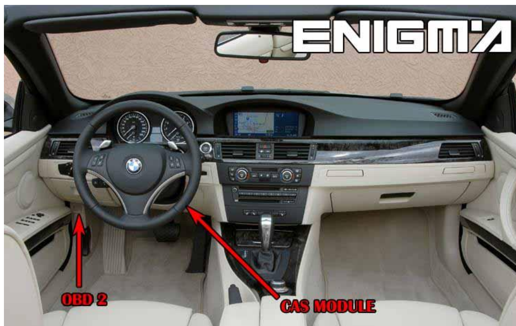
PHOTO 1: Locate the CAS3 module in the car.
