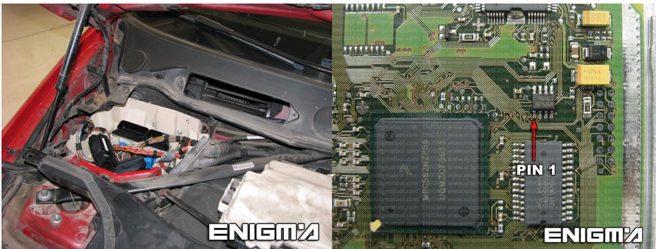
PHOTO 1: Connect cable C4 to EEPROM memory according to the picture above.
