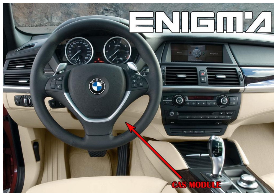
PHOTO 1: Locate the CAS3+ module in the car.
