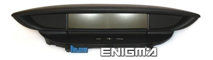
USE CABLE C4, OPEN BOX LOCATED UNDER DASH, PLEASE MAKE IT CAREFULLY, THEN LOCATE EPROM MEMORY 93C46, USUALLY WE DON'T NEED TO DESOLDER IT, AND CLIP IT CHECKING PIN 1 AS SHOWN OF PHOTO BELOW:
